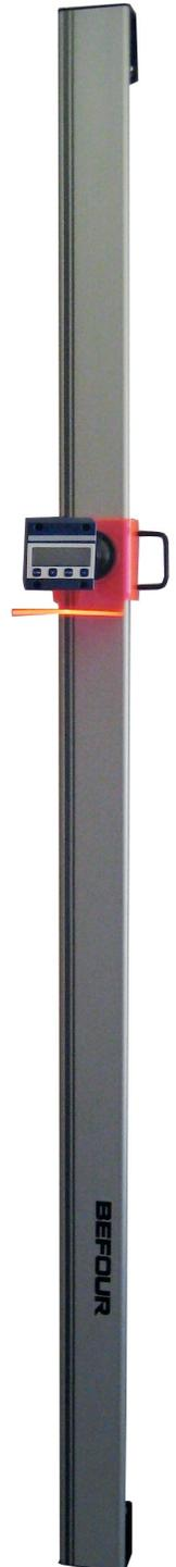
The measurement rail is constructed of attractive anodized aluminum for years of dependable use. The head-piece is constructed in safety-red acrylic with two convenient handles so that the digital stadiometer can be operated from either side. included are a 48" calibration level and all necessary mounting hardware.
